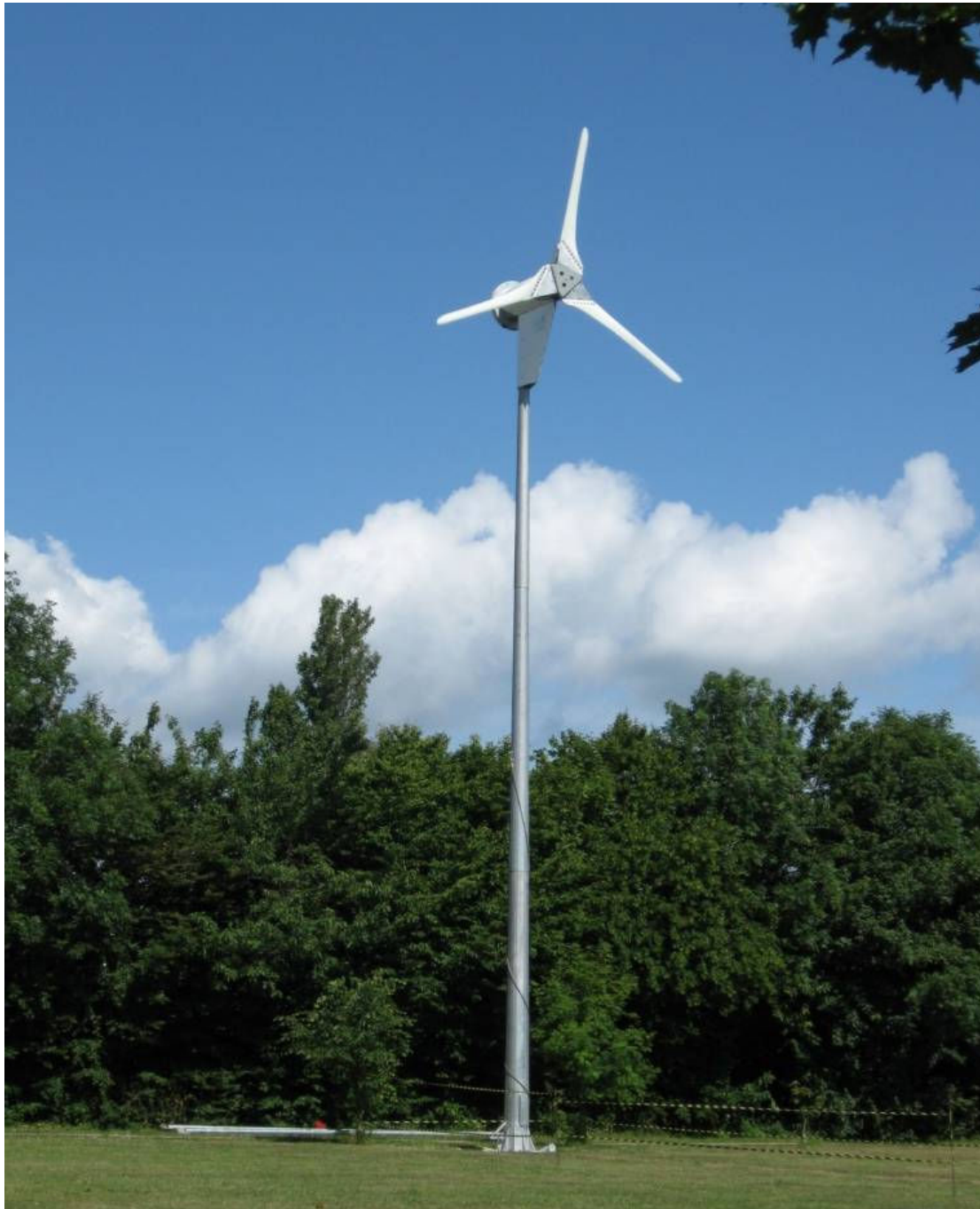
Example: Proven WT6000 wind turbine on 15m mast at Eastchurch CoE Primary School, Sheppey.
